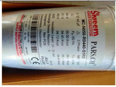
CONCLUSION: Place and date of inspection at Shreem Electric limited located in Kolhapur,India on 14/08/2021 and the sample test performed by manufacturer from 14/08/2021 to 20/08/2021. Sample test witnessed by our SAI inspector in laboratory of the manufacturer and concluded that the goods are in conformity with standard No.: EN 60831-1
