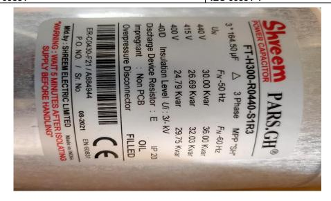
**CONCLUSION:** Place and date of inspection at Shreem Electric limited located in K olhapur,India on 14/08/2021 and the sample test performed by manufacturer from 14/08/2021 to 20/08/2021 Sample test witnessed by our SAI inspector in laboratory of the manufacturer and concluded that the goods are in conformity with standard No.: EN 60831-1 Furthermore, we confirm that the test report is acceptable and the manufacturer's laboratory found to be as qualified. Manufacturer's Representative
