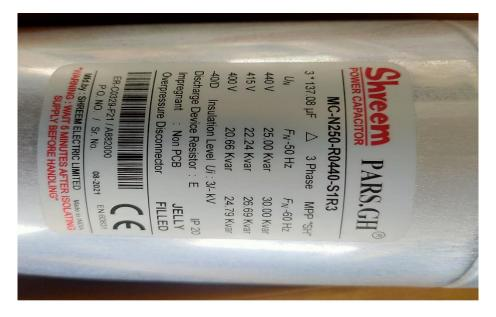
CONCLUSION: Place and date of inspection at Shreem Electric limited located in Kolhapur,India on 14/08/2021 and the sample test performed by manufacturer from 14/08/2021 to 20/08/2021-. Sample test witnessed by our SAI inspector in laboratory of the manufacturer and concluded that the goods are in conformity with standard No.: EN 60831-1
