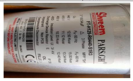
**CONCLUSION:** Place and date of inspection at Shreem Electric limited located in K olhapur, India on 14/08/2021 and the sample test performed by manufacturer from 14/08/2021 to 20/08/2021 Sample test Witnessed by our SAI inspector in laboratory of the manufacturer and concluded that the goods are in conformity With standard No.: EN 60831-1 Furthermore, We confirm that the test report is acceptable and the manufacturer's laboratory found to be as qualified.
